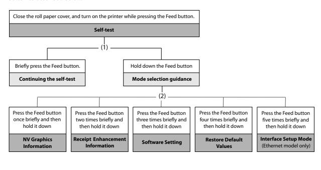
Open the roll paper cover, turn on the printer while pressing the Feed button, and then close the roll paper cover.
