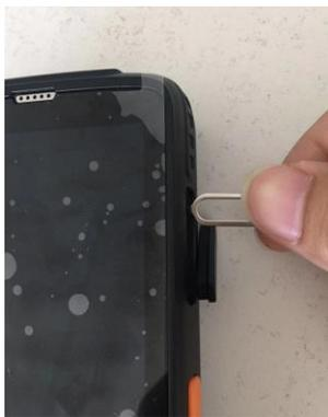
Step 1: Open the cover of SIM/TF card slot.
