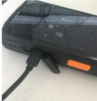
Connect the N7 to a power outlet using the included AC adapter or USB cable.
