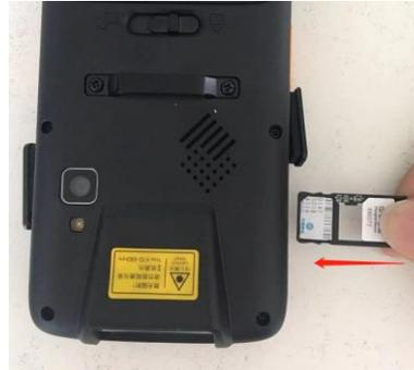
Step 1: Open the cover of SIM/TF card slot and pull the tray out from the slot.
