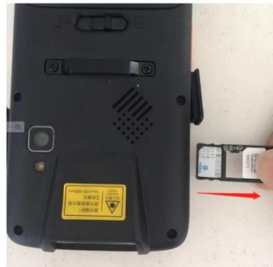
Step 2: Pull the tray out from the slot with the help of retrieve card pin, then remove the SIM/TF card.
