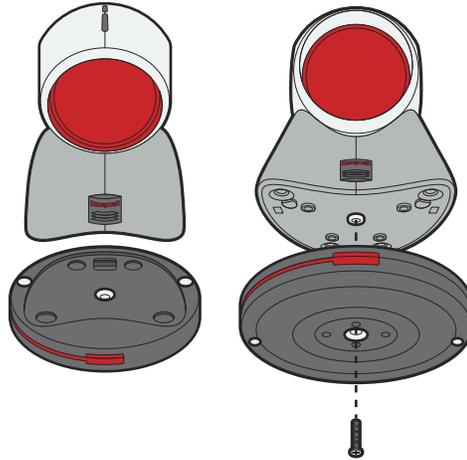
2. Mount the base and scanner to the counter using the 2 wood screws. You may have to rotate the base in order to line up the holes for the screws.
