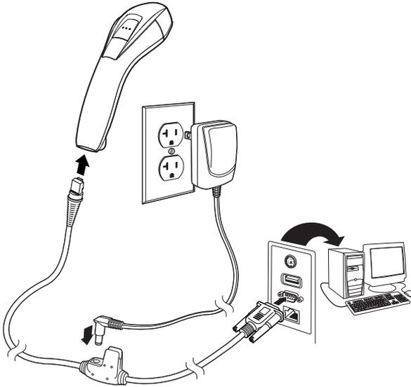
3. Plug the serial connector into the serial port on your computer. Tighten the two screws to secure the connector to the port.
