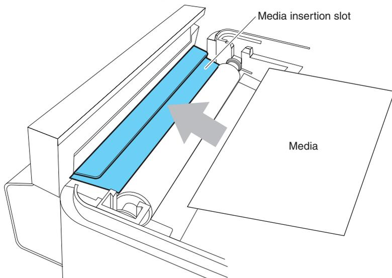
5. Make sure the media is in abutment with the left media guide and then adjust the position of the right media guide in accordance with the media width.
