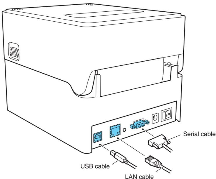
3. Insert the other end of the cable into the appropriate interface port in the host computer.
