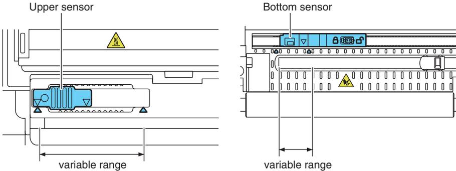
The range of bottom sensor and upper sensor horizontal adjustment is 10 steps between the triangle marks (▲).
