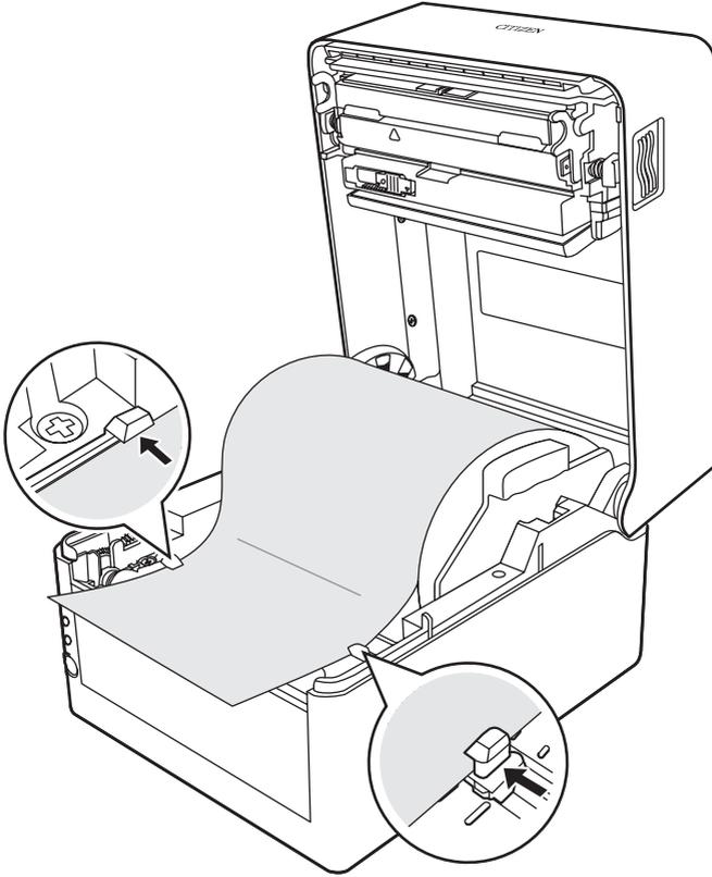
6. Slide the head balance adjustment slider located near the thermal head along the media size scale (inches) so that the position of the notch in the slider matches the media width.
