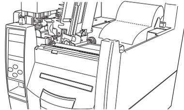
2. Open the rewriter cover and remove the rewriter flange.
