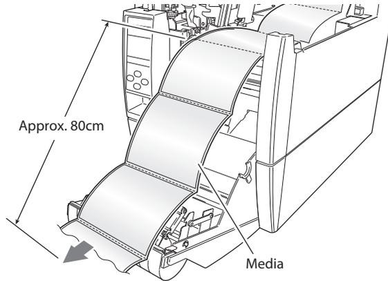
5. Insert the tip of the media through the media enter slit from the external side of rewinder cover.
