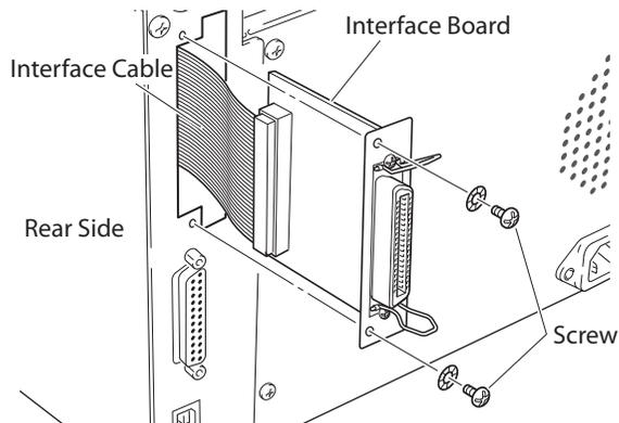
2. Remove the connecting cable from the interface board and reconnect the cable to the connector of the replacement interface board
