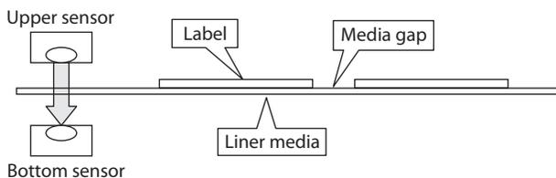
3. If the Pause Key is pressed then released while the MENU key is continually pressed, the sensor is automatically adjusted.
