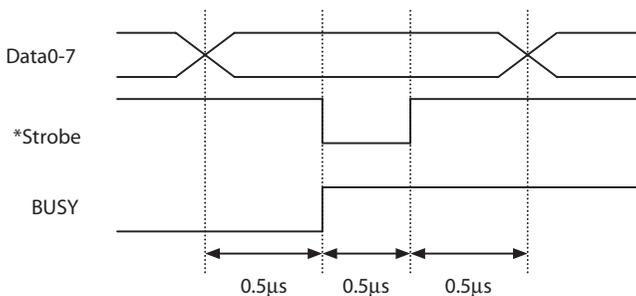
**Note:** Busy rises when \*Strobe signal starts, and data is latched with \*Strobe signal starts.
