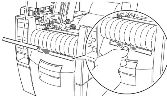
3. Open the rewriter cover and remove the rewriter flange.
