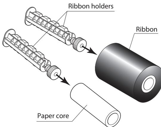
2. Install the unused ribbon and holder in to the rear ribbon drive unit. The splines on the ribbon drive gear mechanism engage with the end of the ribbon holder.
