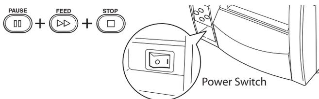
2. After "Sensor Cal Mode" lights up, release the keys to change the printer to sensor adjustment setting mode.
