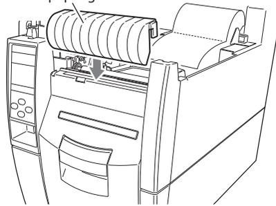
2. Slide the media enter slit cover above the rewriter cover to the left or right while pressing down on its center and remove.
