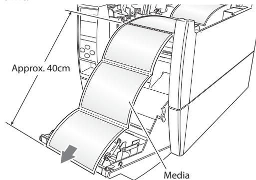
4. Peel off a number of labels at the tip part of the media from the liner so that the liner unit is in contact with the peeler roller when closing the rewriter cover.
