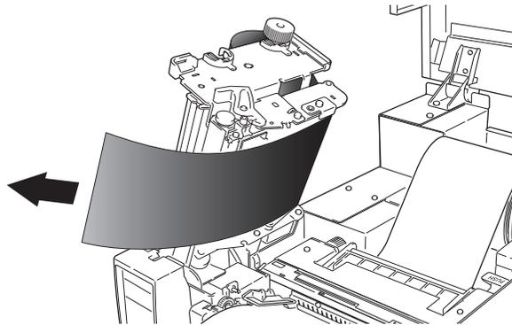
4. Using tape etc., fix the ribbon that you have pulled out on the ribbon holder on which the paper core has been set and wind it on the ribbon holder.
