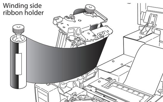
5. Set the ribbon holder on which the paper core has been set in the ribbon drive unit, then rotate it in the direction shown by the arrow to remove slack and wrinkles from the ribbon.
