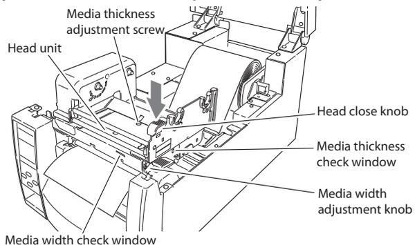
8. With the power switched on, push the FEED key to feed the media. It will halt at the next print start position.
