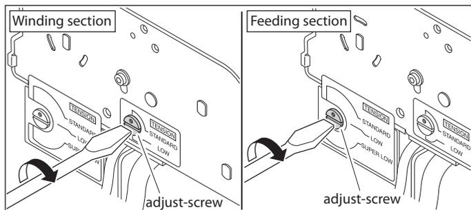
When turning adjust-screw, use a flat-tip screwdriver.
