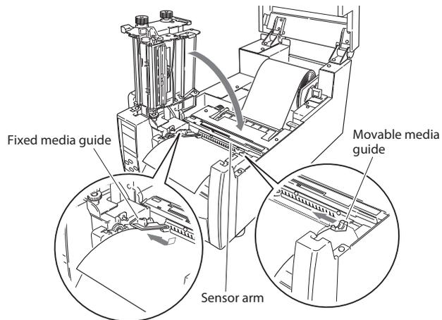
7. Lower the head unit back down to the closed position. Push the head close knob firmly to close and lock the mechanism. The mechanism is only locked correctly when you hear a "click". Align it with the width of the media that has been set, then set the media width adjustment screw and the media thickness adjustment knob. See "Chapter 3 Printer Adjustments".
