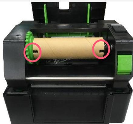
3. Insert the right side of ribbon rewind spindle first. Then, insert the left side to the hole at the left side of ribbon rewind hub (green).
