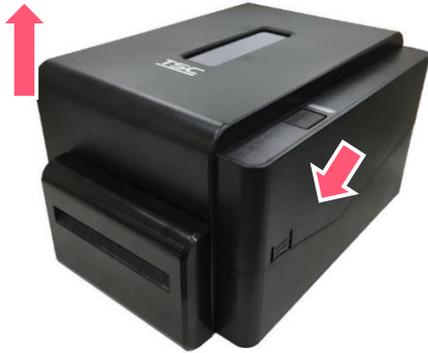
1. Refer to chapter 3.3 to install the label and use software to set the media sensor type and calibrate the selected sensor.
