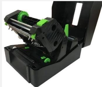
4. Refer to chapter 3.3 to install the label. Use software to set the media sensor type and calibrate the selected sensor. (Please refer to chapter 4,5)
