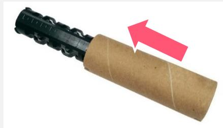
2. Open the ribbon access cover and the media cover. Insert the paper core to the ribbon rewind spindle.
