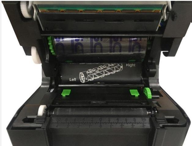
6. Insert the right side of ribbon supply spindle (marked "R") to the ribbon supply hub first. Then, insert the left side of ribbon supply spindle to the hole at the left side of ribbon supply hub (green).
