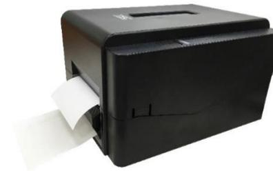
6. Close the media cover and use software to make calibration then enable the peel mode. (Please refer to chapter 4&5)
