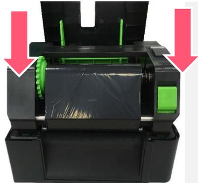
6. Close the print head mechanism with both hands and make sure the latches are engaged securely. Use hardware or software to set the media sensor type and calibrate the selected sensor. (Please refer to chapter 4 & 5.)
