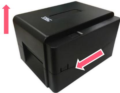
1. Open the printer top cover by pressing the top cover open tabs located on each side of the printer.
