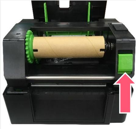
4. Push the print head release button to open the print head mechanism.
