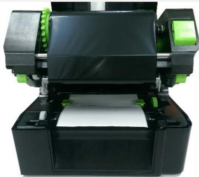
5. Feed the paper, printing side face up, through the media sensor and place the label leading edge onto the platen roller. Move the media guides to fit the label width.
