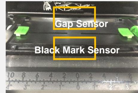
Note: The black mark sensor position is moveable and the gap sensor is fixed. Please make sure the gap or black mark is at the location where media gap/black mark will pass through for sensing.
