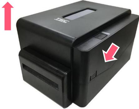
1. Open the printer top cover and refer to chapter 3.3 to install the label.
