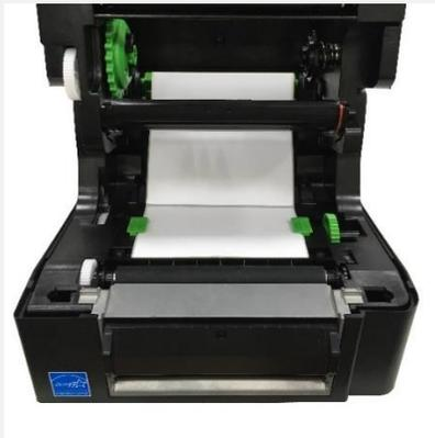
2. Push the print head release button to open the print head mechanism and feed the media through the media sensor. Move the media guides to fit the label width.
