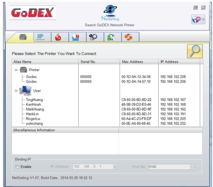
2. There are six tabs on the top of interface which can configure different types of network settings. But for the data security reason, you need correct password to enter the configuration pages.
