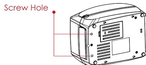
5. Close the printer cover and printing mechanism. Then to turn the printer upside down.
