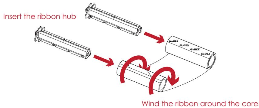
3. A ribbon module is assembled as below.
