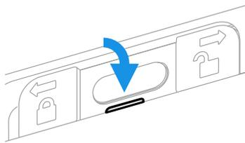
3. Insert the battery (insert the non-connector side first, then press the battery down to establish a connection between the battery and the phone).
