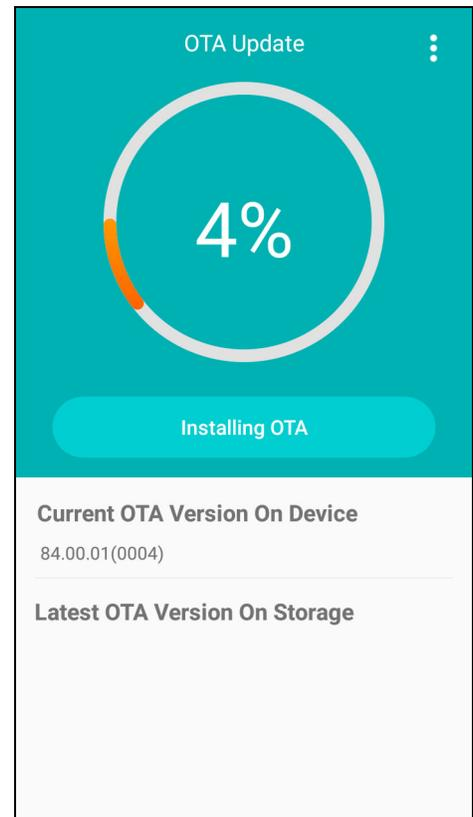
9. Once the installation is complete (100%), select **OK** when prompted to **Reboot** the computer. The computer reboots and finishes the update.
