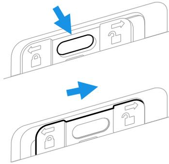
2. Open the battery cover with the battery cover buckle handle
