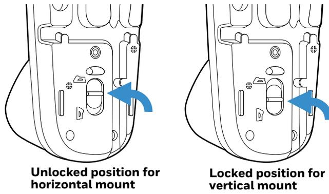
Use 30mm screws, appropriate for the mounting surface material, to mount the base securely.
