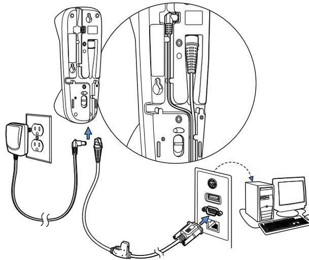
4. Plug the serial connector into the serial port on your computer. Tighten the two screws to secure the connector to the port.
