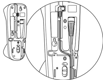
5. Replace with the new cable. Insert the connector into the opening and press firmly. The connector is keyed to go in only one way, and will click into place.
