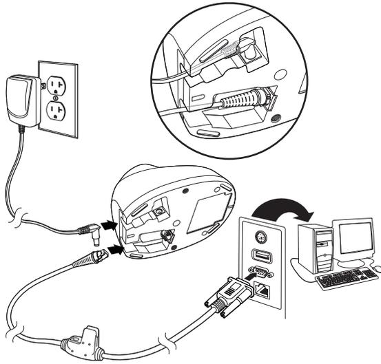
**CCB-H-010BT/CCB-H-010BT-BF Base RS232 Serial Port Connection:**
