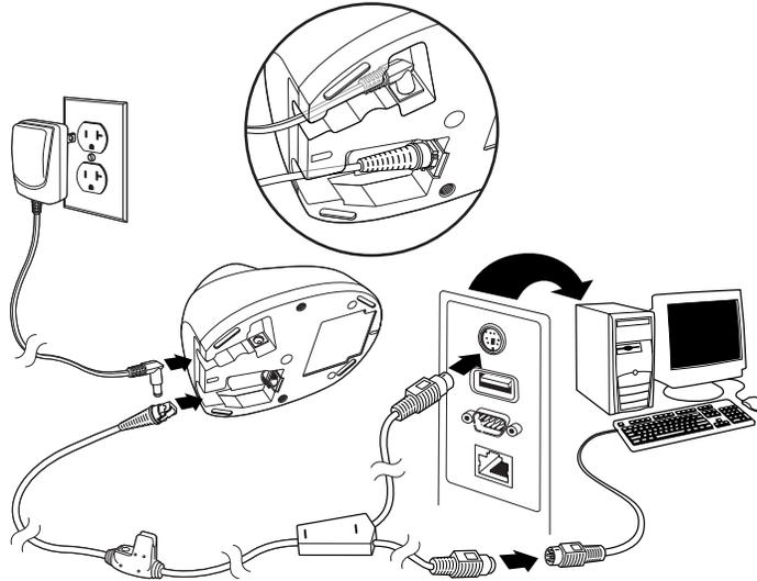
**CCB-H-010BT/CCB-H-010BT-BF Base Keyboard Wedge Connection:**
