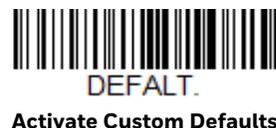
**Note:** *If using a cordless system, scanning this bar code also causes both the scanner and the base or Access Point to perform a reset and become unlinked. The scanner must be placed in its base to re-establish the link. If using an Access Point, the linking bar code must be scanned. See [Cordless System Operation](#) beginning on page 41 for additional information.*
