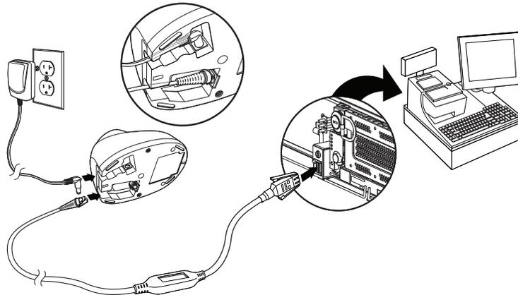
2. Turn the terminal/computer power back on. The scanner beeps.
