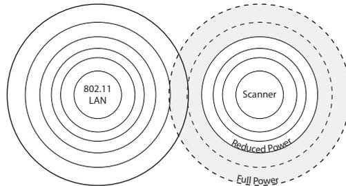
Scan one of the bar codes below to set the scanner's power output to Full Power (100%), Medium Power (35%), Medium Low Power (5%), or Low Power (1%).
