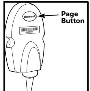
Scan the linking bar code on the top of the Access Point to establish a connection between the Access Point and the scanner. The scanner emits a short beep and flashes the green LED to confirm a connection with the Access Point. The Access Point's Page button remains blue.
