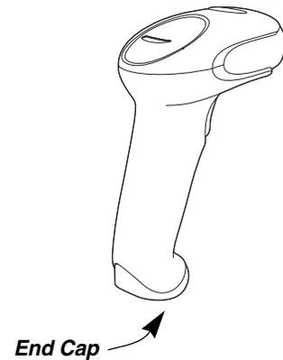
1. Use the hinged wire or a flat head screwdriver to remove the screw from the end cap.
