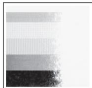
The second sample, left, shows an incorrectly set “media width adjustment”.
