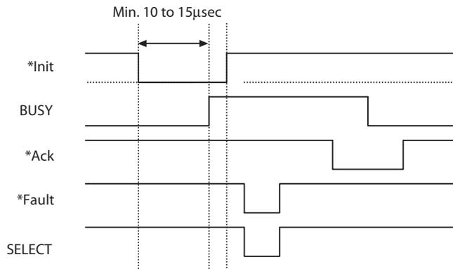
**Note:** If the \*Init signal does not have width of 10 to 15 μsec or more, it cannot act as an Init signal. If it is lower, the \*Init signal is ignored. BUSY starts up when the \*Init signal is perceived.
