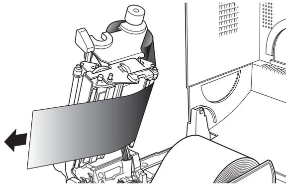
5. Using the adhesive leader of the ribbon or some adhesive tape, fix the ribbon that you have pulled out on the ribbon holder on which the paper core has been set and wind it on the ribbon holder.
