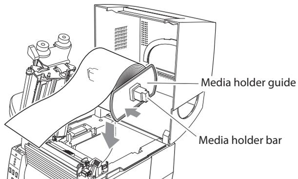
4. Set the media roll and media holder in to the printer as shown above. It is advisable to pull a length of media forwards and through the mechanism ready for later positioning.
