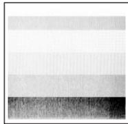
The first sample, left, shows an incorrectly set “media thickness adjustment”. For standard label media, it is recommended you set the blue dial to the “0” position.
