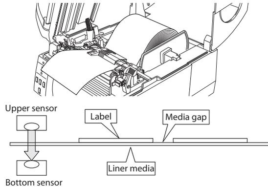
3. If the PAUSE key is pressed and released while the MODE/ REPEAT key is pressed, the PRINT LED goes off, after the CONDITION LED switches from lit to rapid flashing, media feeding starts, and the sensor is automatically adjusted.
