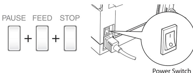
2. After the PRINT LED and CONDITION LED light up, release the keys to change the printer to sensor adjustment setting mode.
