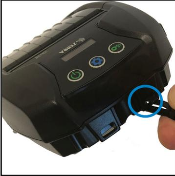
1. Clip one end of the shoulder strap to the post (circled) on the front side of the printer.
