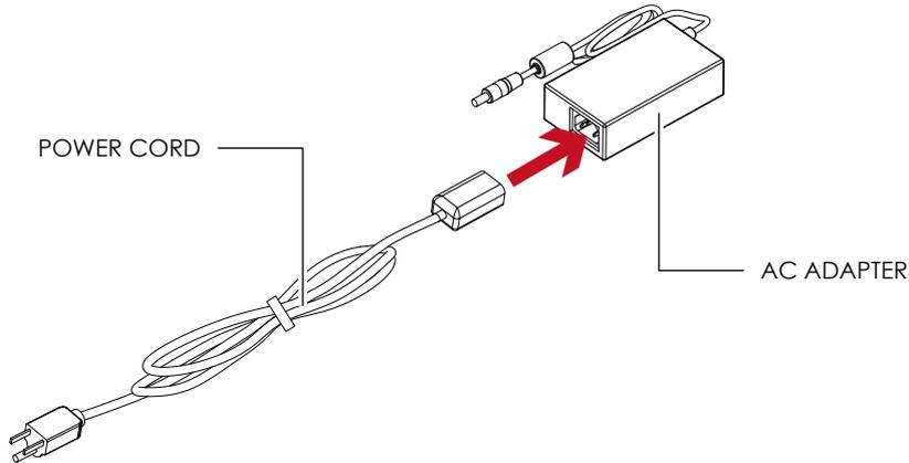
Connect the jack of the power adapter to the printer and connect the plug of the power adapter to the socket of the wall.
