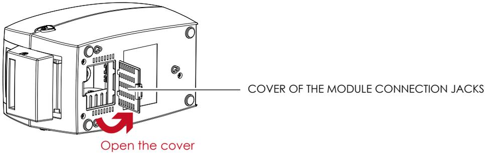
7. Plug the connector for the cutter to the jack.
