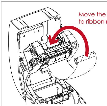
Move the empty ribbon core upward
