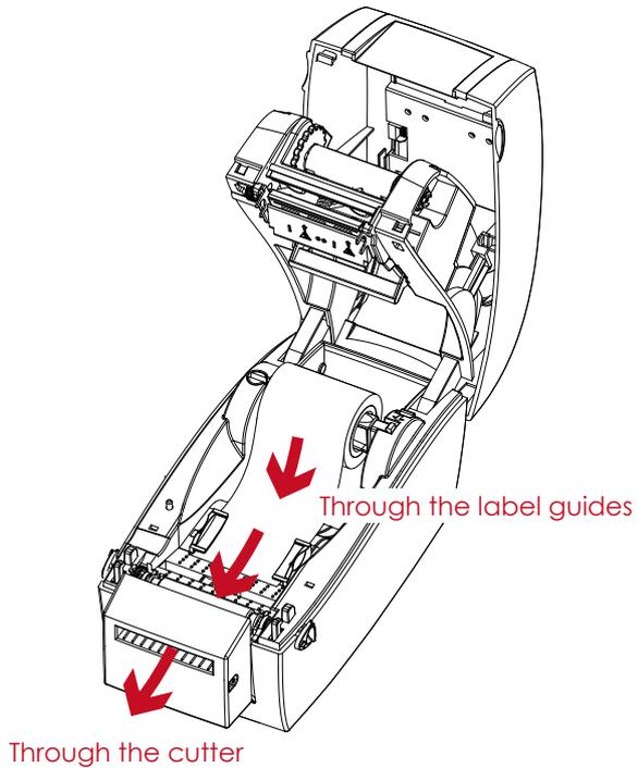
2. Close the top cover and printing mechanism. To finish, press the FEED button to set the label position.
