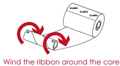
3. A ribbon module is assembled as below.
