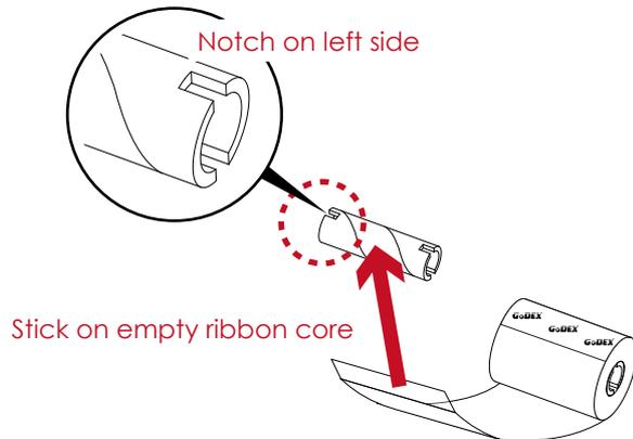
2. Wind the ribbon around the empty ribbon core for 2 to 3 circles.
