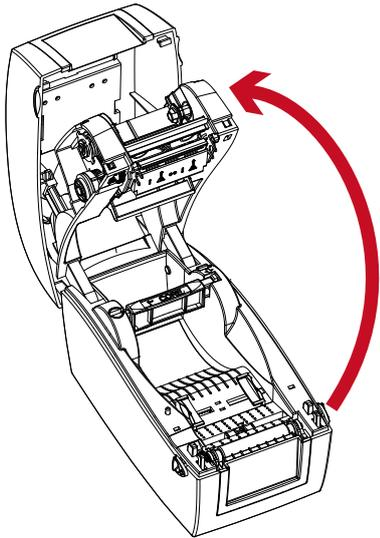
The printing mechanism is lifted up with the printer cover
