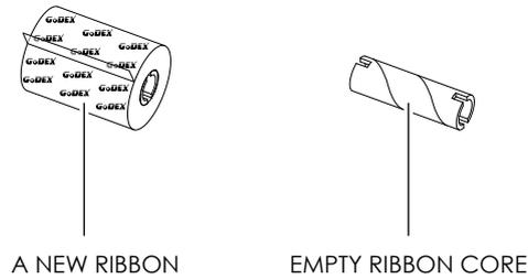
1. Attach the ribbon to the empty ribbon core with the adhesive strip at the end of the ribbon.
